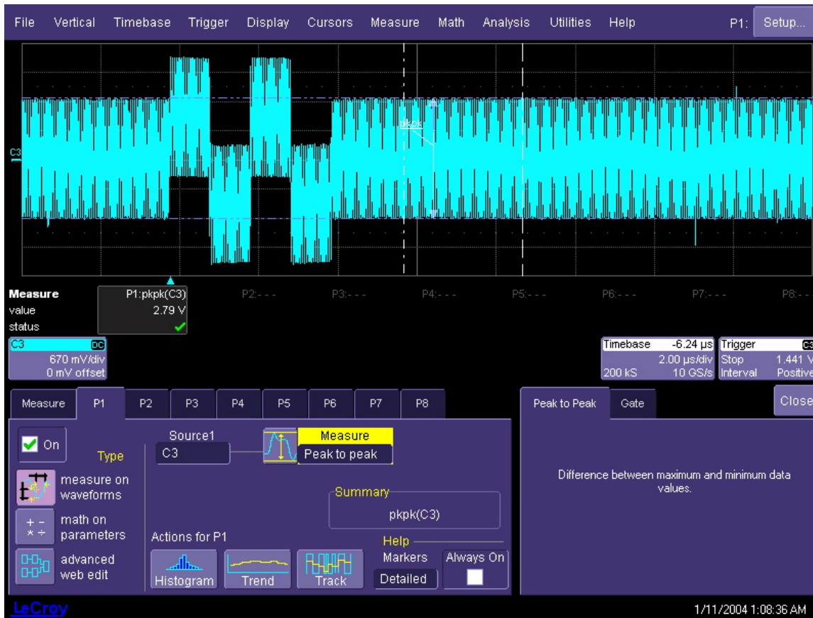
Figure 34: Setting the disturbing signal level for mode 4 test
