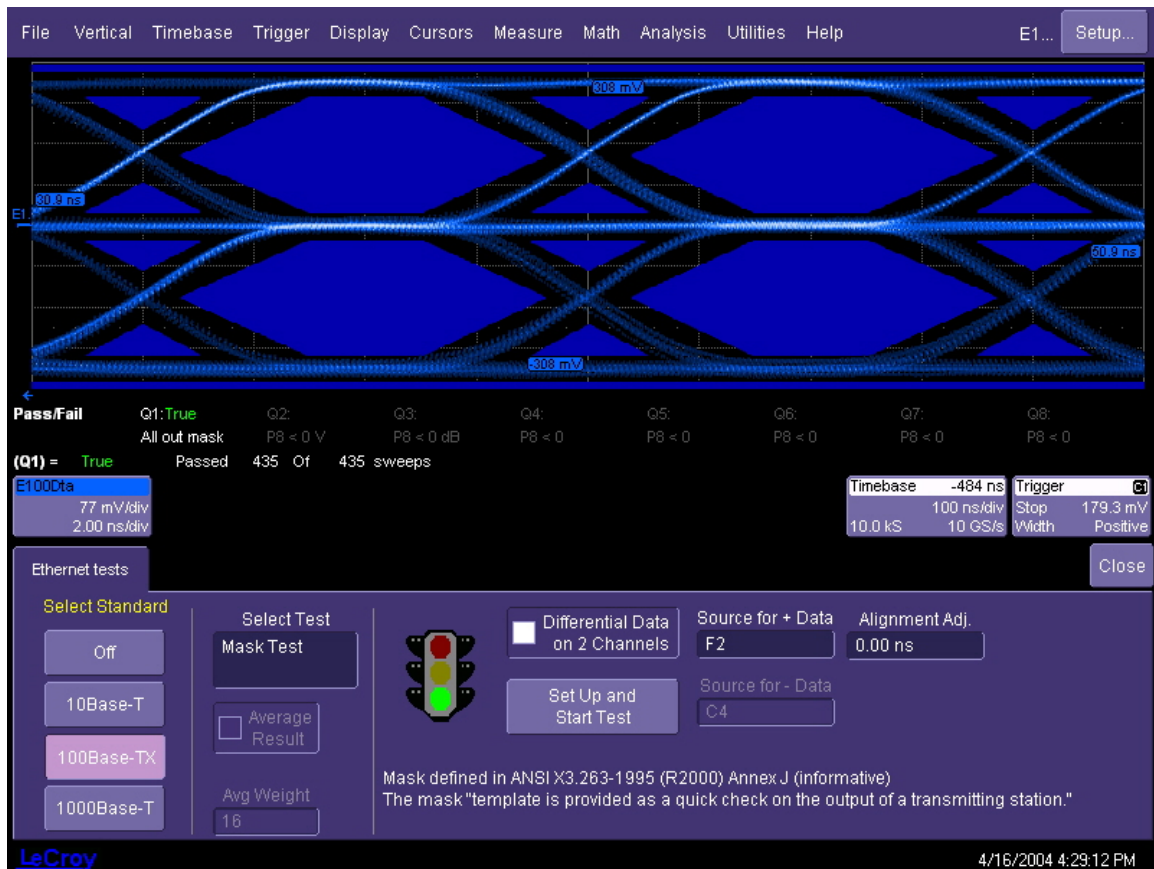
Figure 20: 100Base-TX Mask Test. Note that this display is achieved when the analog persistence display mode is selected
