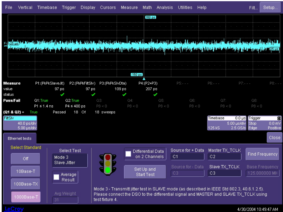
Figure 39: Jitter in slave mode. The trace shows the filtered track of the timing jitter between the master and slave transmit clock signals (TX_TCLK).
