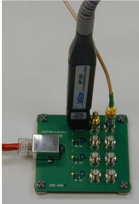
Figure 29: Probe connections for differential output voltage and mask test. The disturbing signal is connected via the SMA cable. The device under test is attached to the RJ45 connector at the left of the picture.
