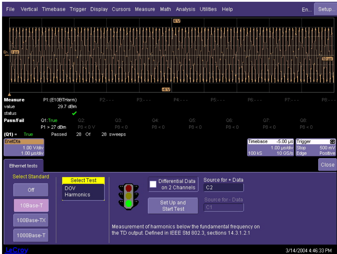
Figure 9: 10Base-T DOV Harmonics
