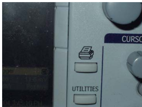
Figure 4: Print Screen button on instrument front panel
